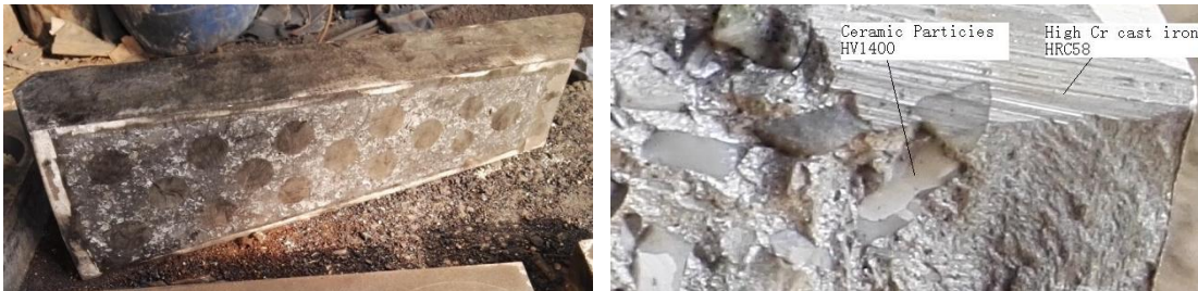
Picture 3-3 Metal Ceramic Composite Liner (HP863 Liner of High Cr cast iron +ZTA ceramic)
