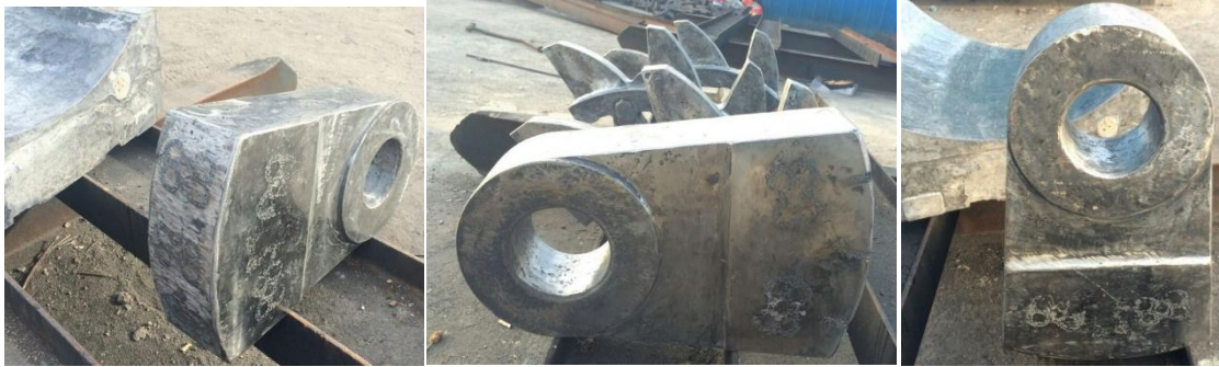
Picture -2 Hammer of Martensite steel and ceramic composite-external view
